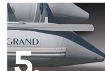
5. Extended and lowered down tube ends are an excellent feature for more flotation and stability
