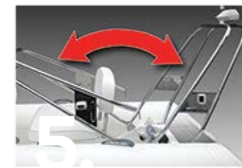
5. New folding stainless steel navigation arch for compact storage and the occasional low bridge
