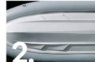
2. The unique 4-step hull is fast and economical (S300 and S330 only)
