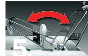
5. New folding stainless steel navigation arch for compact storage and the occasional low bridge
