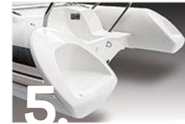
5. GRP step ends with easy access for boarding, swimming and an improved ride
