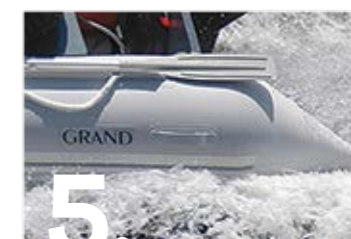
5. Lowered tube ends stabilize the boat at fast speed and make the ride dry
