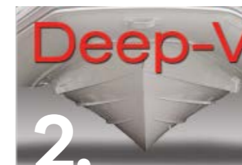
2. Deep-V hull with transom extensions for superior performance and soft ride.
