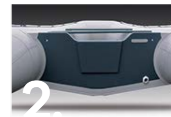
V-shaped transom with original metal reinforced installation system
